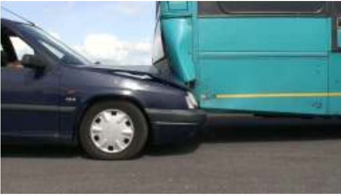
Figure 16 Impact Sequence (Max. Engagement)
